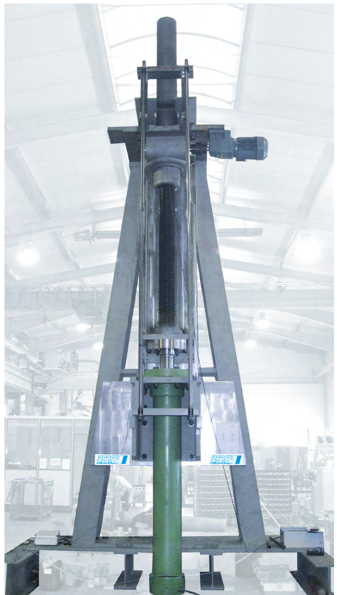
Test configuration for trialling a 200 tons screw jacks type SHE 200.1 before use in a pot lifting system
